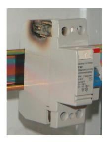
This component is one of the key elements protecting against electric shock. Due to the current flow through the protection device, the mechanical stress on the terminals causes minute loosening of the screws, the consequence of which are sparks which can lead to complete destruction of the unit (the danger of fire increases), reducing your and the building's protection.
